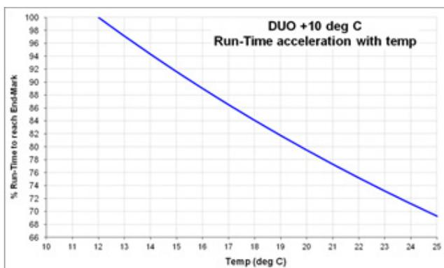
The y-axis represents the actual run-time of the liquid at different temperatures, and is expressed as a percentage of the specified run-out time at an isotherm of 12°C/54°F. So, at an isothermal temperature of 12°C, the liquid dye will reach each time-marker (3, 8, 14 days) within these times +/-15% in time. However, if for example the product is exposed to an isotherm of 21°C/70°F the dye will reach each time marker within only 77% of the intended run-time. In other words, it will reach the;
